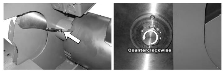
4. Remove old blade and put new one on over the drive pin (below left) and arbor shaft. Be sure to follow the blade rotation arrow (below right).
