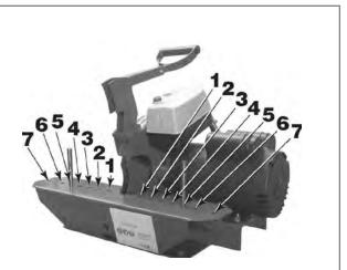
\*This guide only "suggests" the best possible pin placement, as there are variables such as new or used hose, brands of hose, braided or spiral wire reinforcement (4 or 6 wire multi-spiral). As an operator you will learn the best pin placement for the hose you are cutting. Remember that the cut hose should be square and clean.
