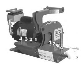
\*This guide only "suggests" the best possible pin placement, as there are variables such as new or used hose, braided or spiral wire reinforcement (4 or 6 wire multi-spiral). As an operator you will learn the best pin placement for the hose you are cutting. Remember that the cut hose should be square and clean.
